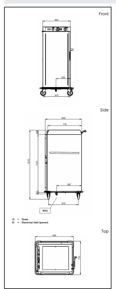
**Electric Supply voltage:** 230 V/1N ph/50/60 Hz
